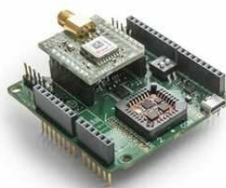
Figure 2: Xsens MTi-7 integrated into Development Kit, and specifications
