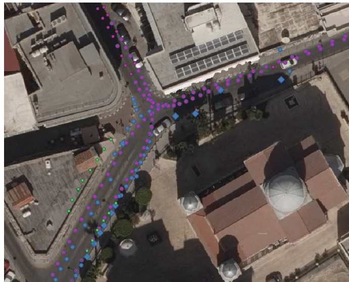
Figure 12: Visualization of solutions provided by RTK Lib (blue), F9P (magenta) and GrafNav (green)
