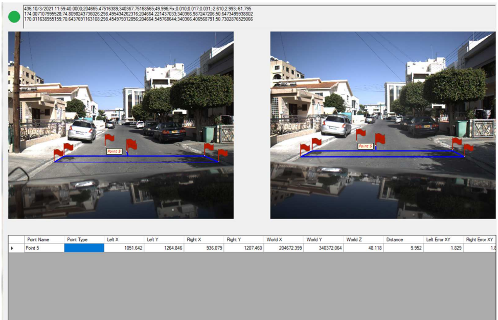
Figure 25 : Points, lines and polylines measured in a frame pair
