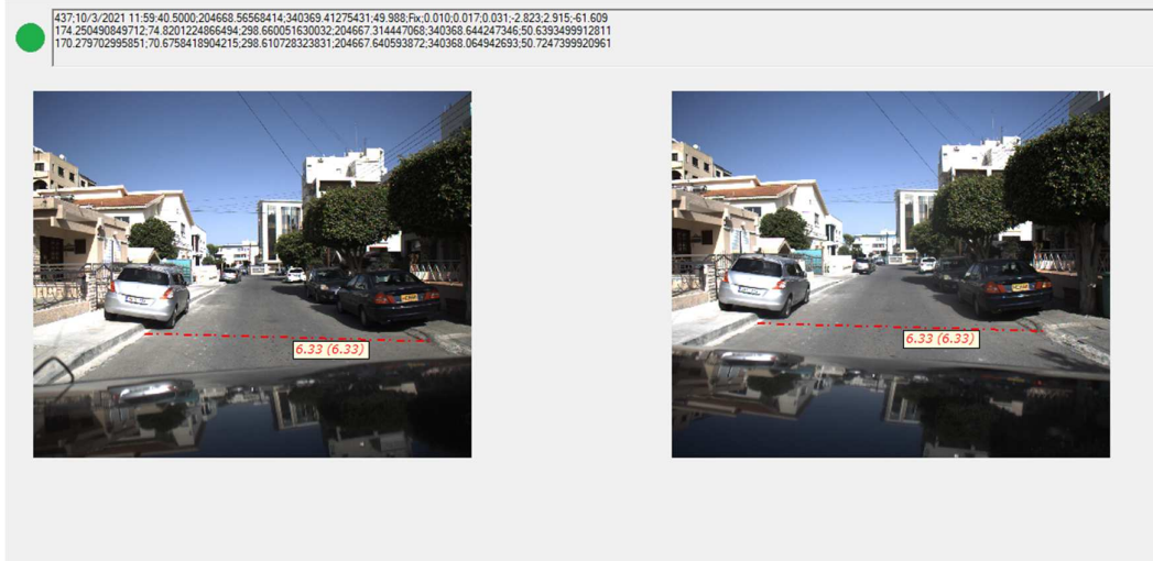
Figure 26 : Distance measurement displayed on both left and right frames. The measurement is given in meters.
