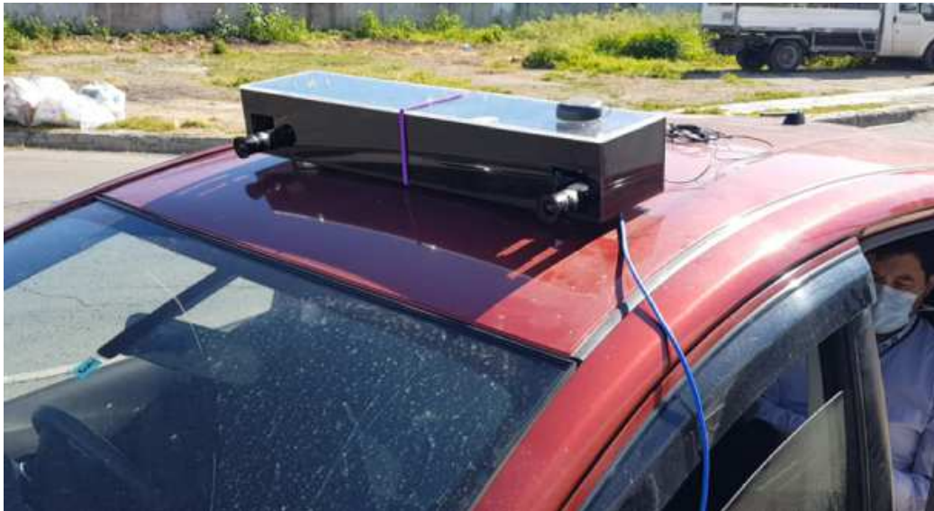
Figure 9: MOBILO carrier mounted on top of a vehicle
